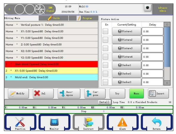
Controller can set four fixtures and two sucker action, clicking the button to be controlled and the indicator turns red when output. Then click on the left so that it becomes  $\sqrt{}$ , clicking "Insert" the action step is inserted into the front steps of the selection procedure.
