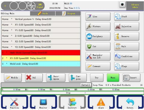
Servo action, Stack action, Fixture action, Injection, Auxiliary action, Reserve action, Check action, Wait action, Series action, Periphery are included in "Teach" button. Clicking those buttons to edit a program. Press "Teach" to back to menu.
