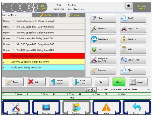
Six steps of [Home] status above, which are default steps status in a new program, can just be edited by click "Edit" to modify the starting position, operating speed and delay time of axes, not be deleted.
